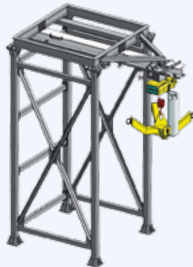
Option: Big bag unloading - with big bag sleeve closing valve
